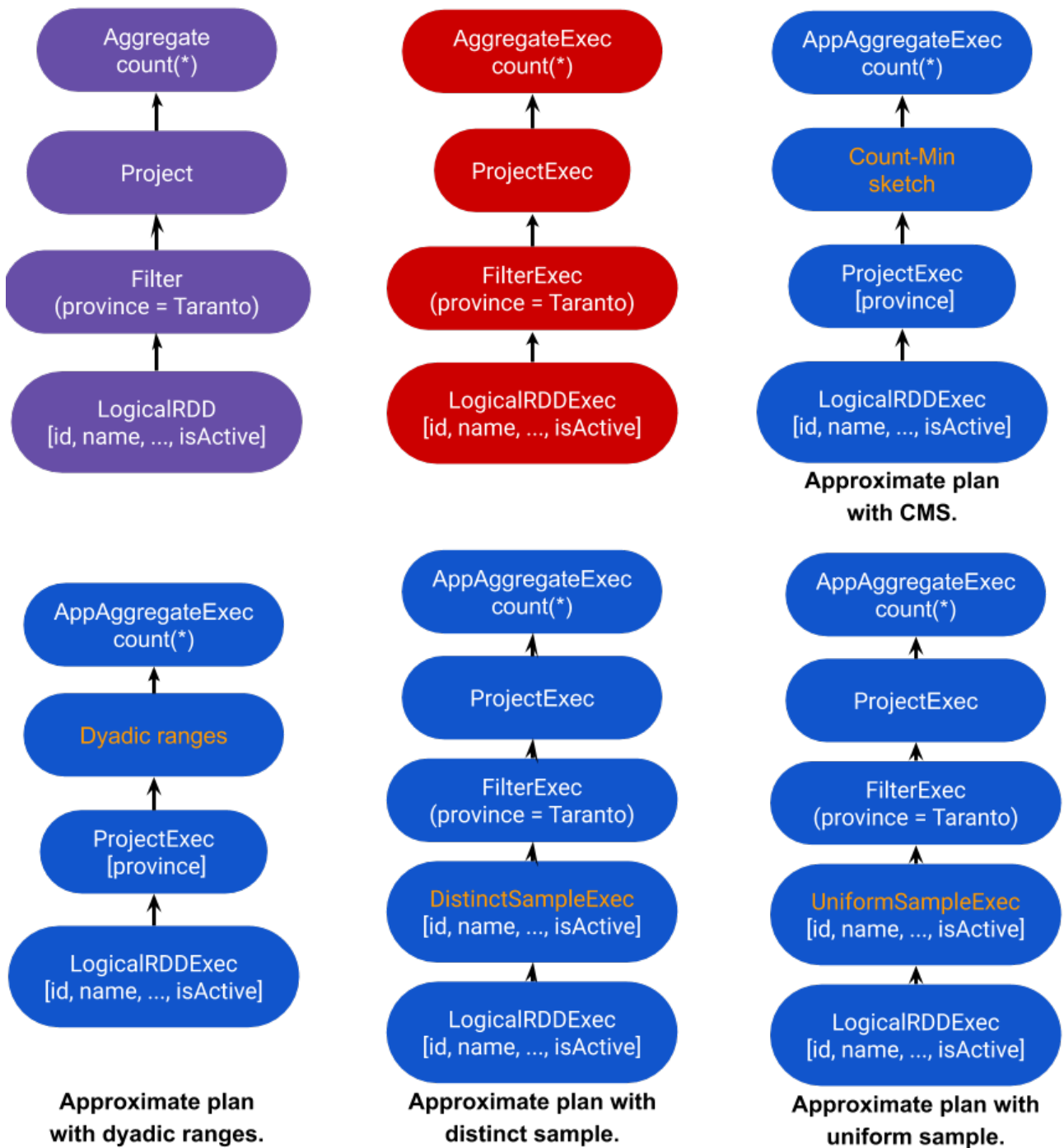
Figure 7: Logical plan (purple) and its candidate physical plans (exact plan is depicted as red, and approximate plans are blue, with the approximate operators noted with orange fonts).
